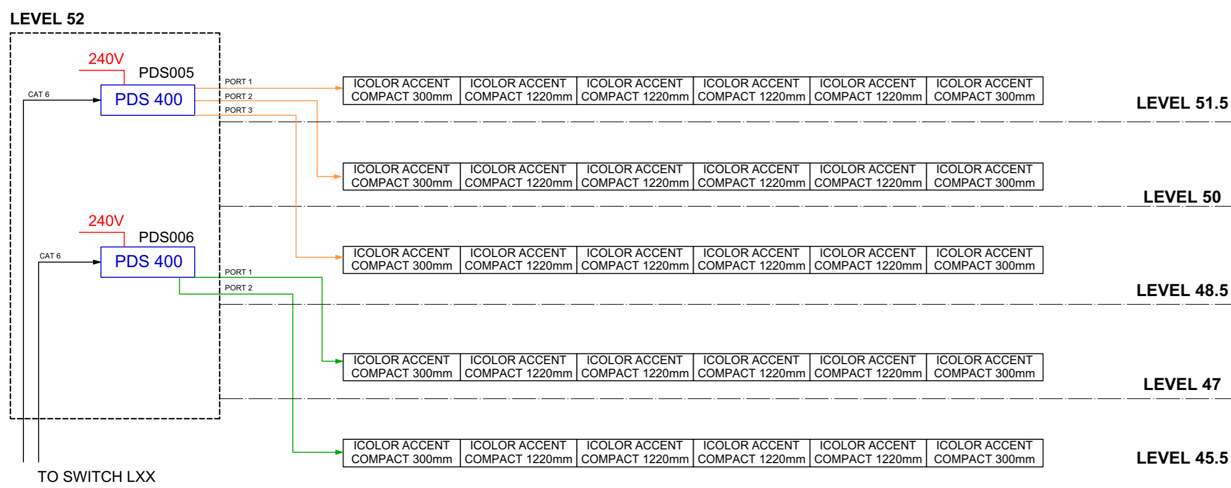
3 SOUTH BUTTRESS - CONTROL SCHEMATIC NOT TO SCALE
