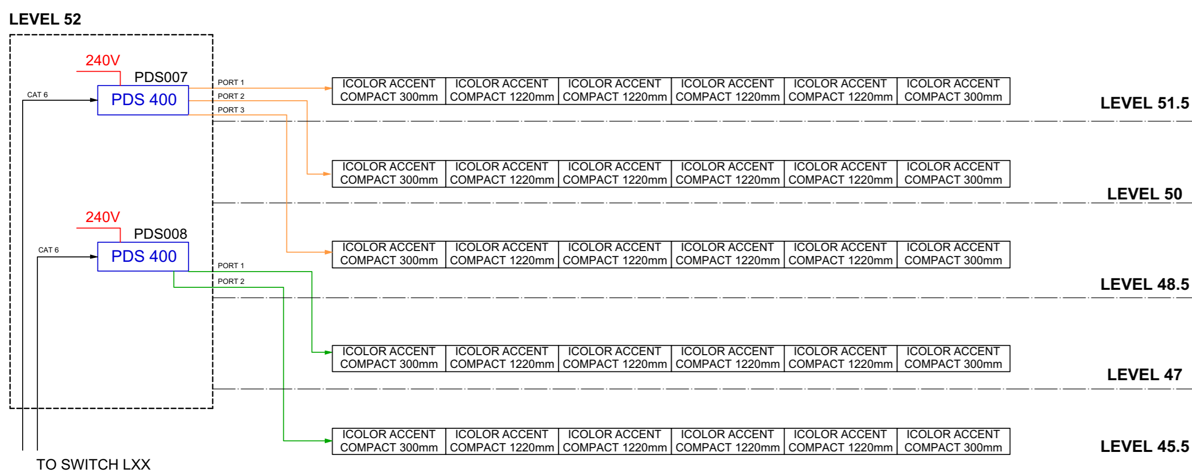
4 WEST BUTTRESS - CONTROL SCHEMATIC NOT TO SCALE
